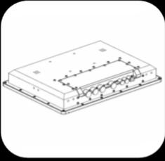
Re-install the cover with all 17 screws for water protection. Only special designed cable with matching waterproof plastic molding should be used.
