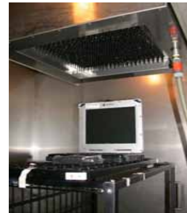
RAIN TEST IP-54
