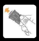
Attach the D-Sub 15-Pin connector to your computer's analog VGA output connector
