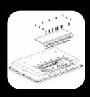
Waterproof Cover: Remove 9 short screws and 8 long screws on this cover to install the cable(s) you need.
